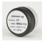
After sampling is complete, the passive sampler is analysed via ion chromatography. The analysis method is validated according to EN 13528 [1], and the laboratory is accredited under ISO/IEC 17025.
