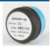
The sampler operates based on the principle of passive diffusion: O<sub>3</sub> molecules enter the housing and are bound to an absorbent medium. Sampling occurs autonomously over 1 to 4 weeks. An integrated protective filter reduces environmental influences such as wind, allowing for precise measurements.
