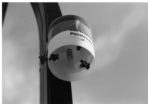
Protective shelter for ORSA5 Sampler in combination with \text{NO}_2 diffusion tube
