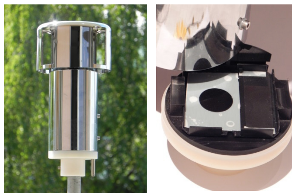
SIGMA-2 sampler for particulate matter and adhesive plate inside the sampler
