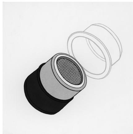
Schematic view of  $\text{NH}_3$  sampler
